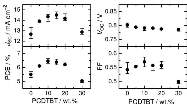
**Fig. 3** Photovoltaic parameters ( $J_{SC}$ ,  $V_{OC}$ , FF, and PCE) of PBDTTT-EF-T/N2200 binary and PBDTTT-EF-T/N2200/PCDTBT ternary BHJ solar cells with different amounts of PCDTBT loading. Each value is an average over a minimum of 10 devices.
