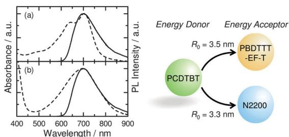
**Fig. 5** (a) The absorption spectrum of PBDTTT-EF-T neat film (broken line) and the PL spectrum of PCDTBT neat film (solid line). (b) The absorption spectrum of N2200 neat film (broken line) and the PL spectrum of PCDTBT neat film (solid line). The strong overlap between the PCDTBT PL and the absorption bands of PBDTTT-EF-T and N2200 gave a Förster radius ( $R_0$ ) of 3.5 nm and 3.3 nm, respectively (ESI,† Fig. S3)
