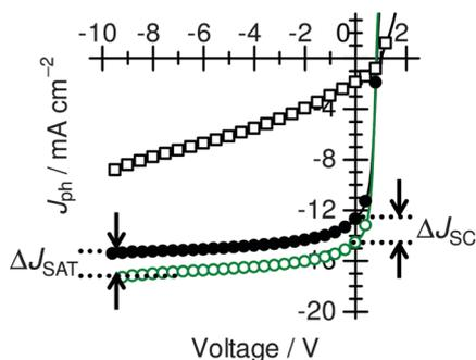
Fig. 6 Photocurrent density  $J_{ph}$  of the binary (solid circles) and ternary (open circles) blend solar cells as a function of the applied reverse voltage measured under AM1.5G illumination ( $100 \text{ mW cm}^{-2}$ ). The loading amount of the PCDTBT was 10 wt%. The  $J_{ph}$  values were obtained by subtracting the current density in the dark  $J_D$  from that under illumination  $J_L$  as  $J_{ph} = J_L - J_D$ .
