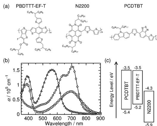
**Fig. 1** (a) Chemical structures of PBDTTT-EF-T, N2200, and PCDTBT. (b) Absorption coefficients  $\alpha$  of PBDTTT-EF-T (circles), N2200 (squares), and PCDTBT (triangles) measured in neat film spin-coated from chlorobenzene. (c) Energy level diagram for neat films of each polymer. The HOMO levels were determined by photoelectron yield spectroscopy, whereas the LUMO levels were estimated by adding the optical energy gap calculated from the 0–0 transition to the HOMO energy (ESI,† Fig. S1).
