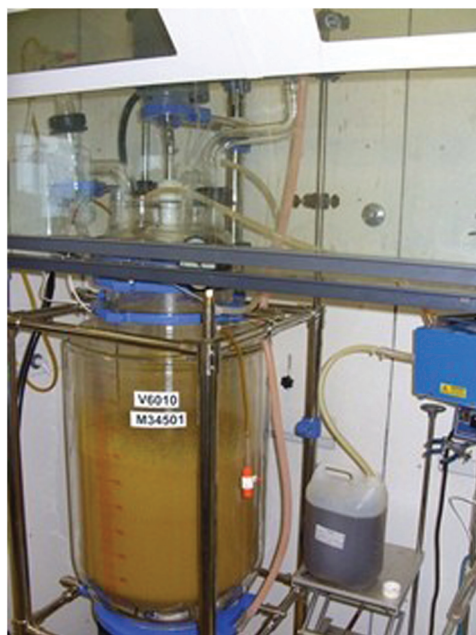
Fig. 11 100 L production of 1SRT-CPO-27(Zn).
