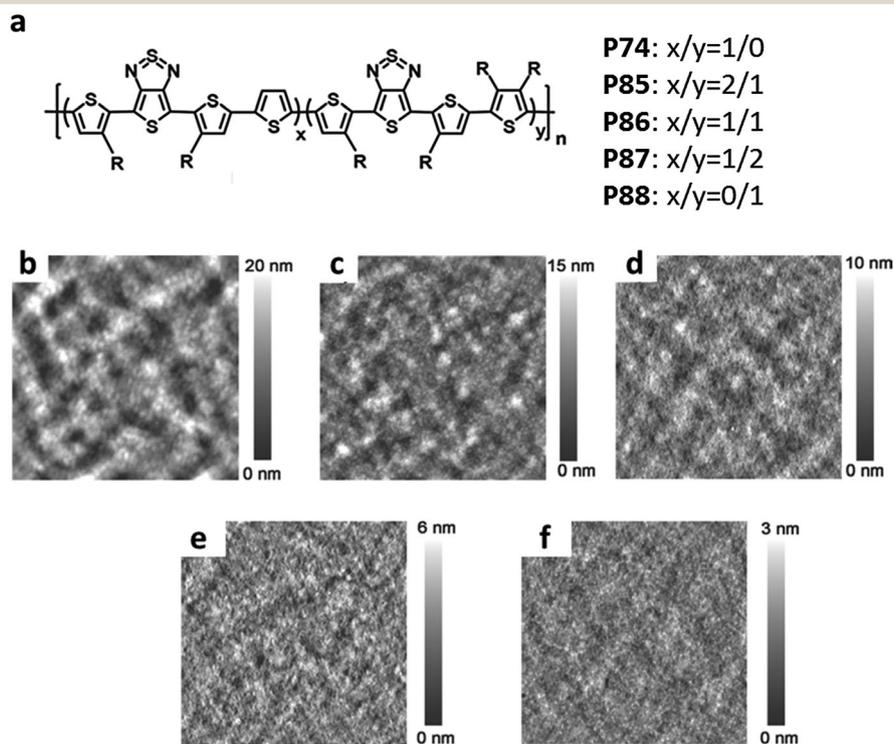
**Fig. 16** (a) Side chain engineering of P74; (b–f) AFM images of P74:PCBM, P86:PCBM, P87:PCBM, P77:PCBM and P89:PCBM, respectively (ref. 135). (From Ji Qi *et al.*, *Adv. Funct. Mater.*, Copyright © 2014 by John Wiley & Sons, Inc. Reprinted by permission of John Wiley & Sons, Inc.)
