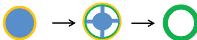
Fig. 9 Hollowing by the Kirkendall effect.
