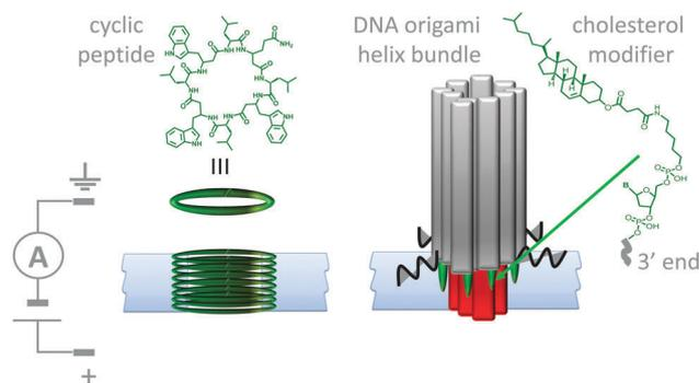
Fig. 11 Artificial nanopores in lipid bilayer membranes made using cyclic peptides (left)<sup>29</sup> and DNA origami (right).<sup>30</sup>
