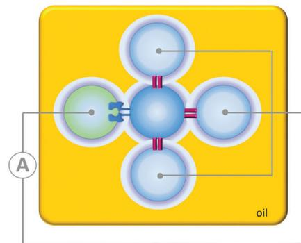
Fig. 24 A simple circuit constructed from a droplet interface bilayer network connected by an  $\alpha$ -haemolysin pore and bacteriorhodopsin.<sup>48</sup>
