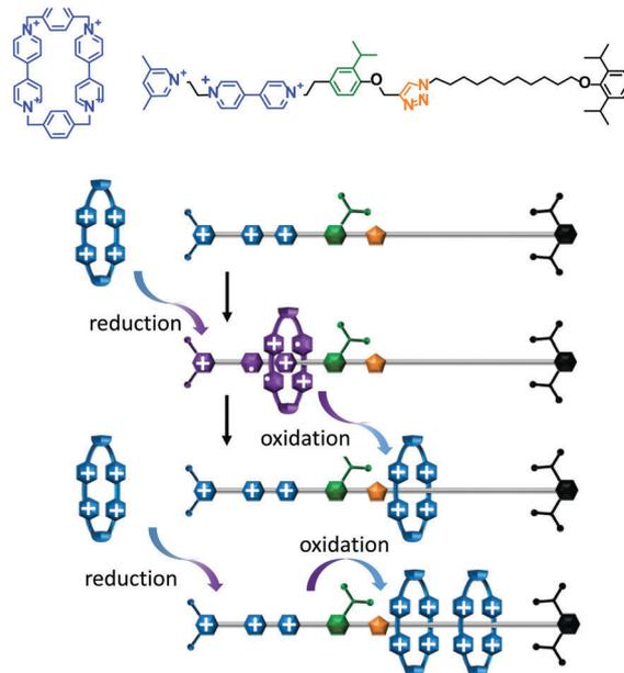
Fig. 4 An artificial molecular pump driven by external switching of redox conditions.<sup>25</sup>
