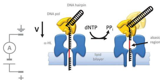
Fig. 20 Polymerase-catalysed replication of DNA monitored at the single-molecule level using a nanopore.<sup>42</sup>
