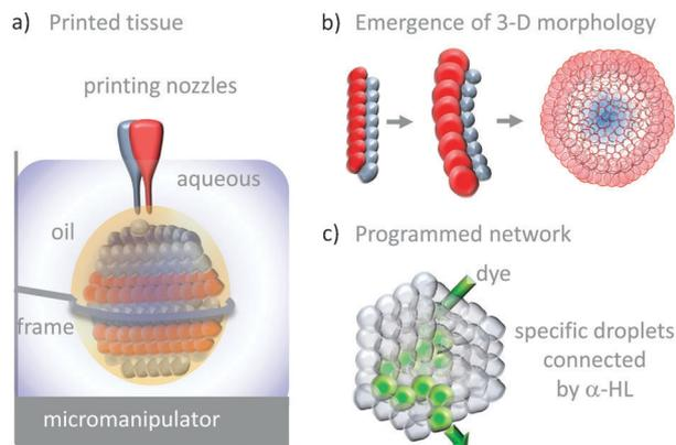
Fig. 26 Tissue-like 3-D printed droplet networks.<sup>50</sup>
