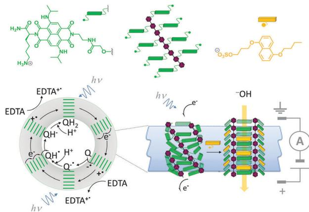
Fig. 16 A self-assembled synthetic transmembrane electron pump that can also open in response to ligand binding.<sup>35</sup> EDTA = ethylene diamine tetraacetate, Q = quinone.
