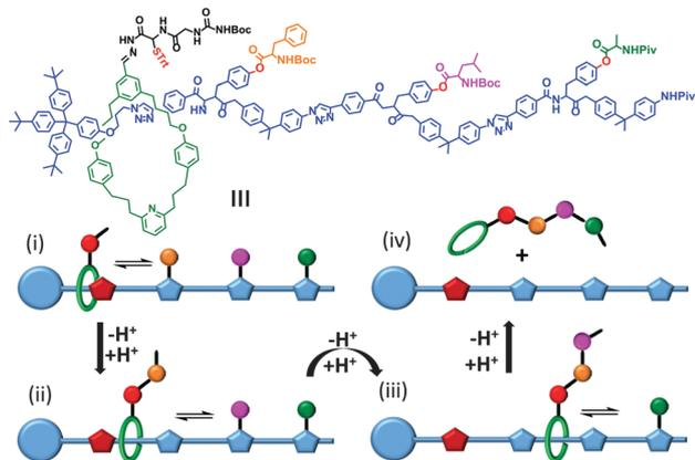
Fig. 3 A rotaxane-based peptide synthesiser.<sup>8</sup> Trt = CPh<sub>3</sub>, Boc = CO<sub>2</sub>t-Bu and Piv = OCOt-Bu.
