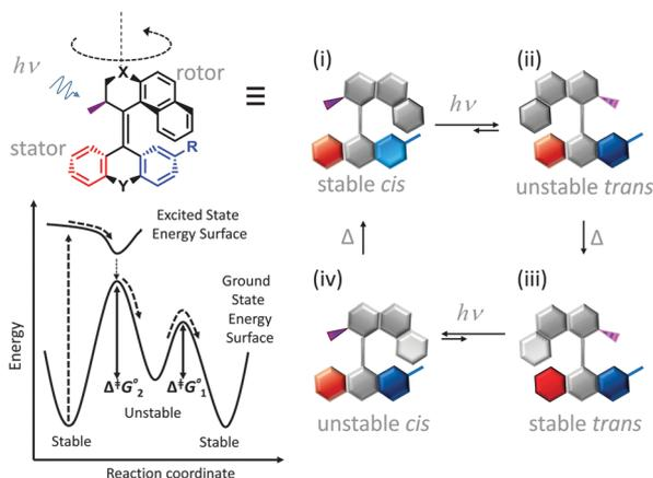
Fig. 8 Light-driven unidirectional intramolecular rotation of a synthetic molecular motor.<sup>9</sup>
