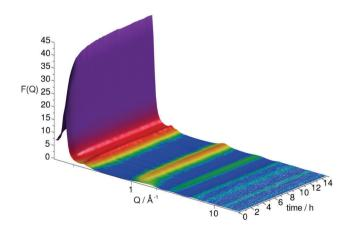
Fig. 5 Evolution of total scattering structure factor over the course of the toluene- $d_8$  hydrogenation under 150 mbar  $D_2$ .
