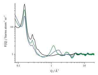
Fig. 3 Total scattering structure factors measured for evacuated 3 wt% Pt/MCM-41 catalyst (black line), for catalyst filled with toluene- $d_8$  by capillary condensation (blue line) and catalyst after 15 h of reaction (green line). An offset of 1 has been applied to all datasets.
