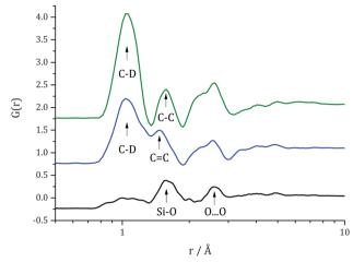
Fig. 4 Direct Fourier transform D(r) of data shown in Fig. 3, i.e. radial distribution function for evacuated catalyst (black line), catalyst filled with toluene- $d_8$  (red line), and catalyst after 15 h of reaction (blue line). An offset was used for clarity.
