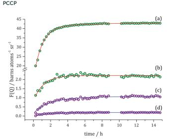
**Fig. 6** Slices taken through evolution of F(Q) (Fig. 5) at specific Q values (symbols): (a)  $Q = 0.15 \ {\rm \AA}^{-1}$ , (b)  $Q = 0.27 \ {\rm \AA}^{-1}$ , (c)  $Q = 1.18 \ {\rm \AA}^{-1}$  and (d)  $Q = 2.90 \ {\rm \AA}^{-1}$ , and exponential fits to the data (solid lines). Green colour indicates changes in Bragg scattering and violet – in diffuse scattering over the course of the hydrogenation reaction.
