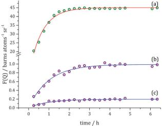
Fig. 7 Changes of F(Q) over the course of toluene- $d_8$  hydrogenation by 250 mbar  $D_2$  at specific Q values (symbols): (a)  $Q = 0.15 \text{ Å}^{-1}$ , (b)  $Q = 0.15 \text{ Å}^{-1}$ 1.18  $\text{Å}^{-1}$  and (c)  $Q = 2.91 \, \text{Å}^{-1}$ , and exponential fits to the data (solid lines).
