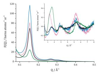
Fig. 2 Two sets of total scattering structure factors for evacuated catalyst (blue and black lines), and catalysts loaded with reagent. Black line indicates an empty catalyst that was later filled with toluene- $d_8$  (green line), whereas blue line presents diffraction from empty catalyst later loaded with toluene- $h_8$  (pink line).
