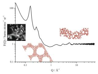
Fig. 1 Total scattering structure factor obtained for evacuated MCM-41 on NIMROD. In a single measurement information about the size and shape of sample's grains can be obtained (low Q-range), as well as unit cell size from Bragg scattering features and interatomic correlations within the sample such as average distances between silicon and oxygen in MCM-41 (high Q-range)
