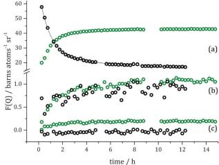
Fig. 8 Changes of F(Q) over the course of toluene- $h_8$  (black symbols) and toluene- $d_8$  (green symbols) hydrogenation by 150 mbar  $D_2$  at specific Qvalues: (a)  $Q = 0.15 \text{ Å}^{-1}$ , (b)  $Q = 1.18 \text{ Å}^{-1}$  and (c)  $Q = 2.90 \text{ Å}^{-1}$
