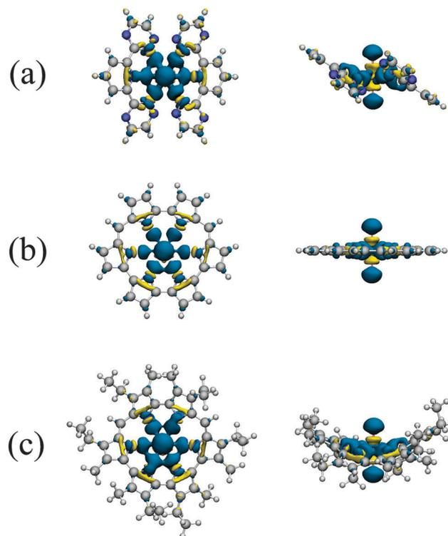
Fig. 6 Electron density differences in (a)  $[\text{UO}_2(\text{BTP})_2]^{2+}$ , (b)  $\text{UO}_2\text{IA}$  and (c)  $\text{UO}_2\text{IA}'$  upon complexation. Blue regions indicate charge accumulation and yellow areas charge depletion. All densities visualised using an isosurface of  $\rho = 0.005$  a.u.
