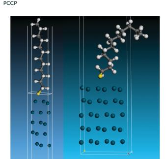
**Fig. 7** Structures used to model the adsorbed thiolate on Pd(111). Left: All-*trans* thiolate. Right: Thiolate with *qauche* defects.
