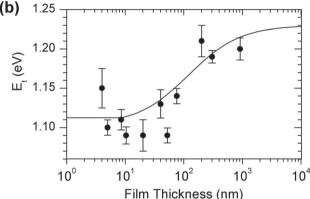
Fig. 4 (a) A plot of the conductivity vs. film thickness for different temperatures. The conductivity increases as the film thickness is reduced, up to a limiting value. The fit of the model discussed is represented with solid lines, and fits the experimental data well. (b) A plot of the total activation energy  $E_{\rm t}$  of the films vs. film thickness. Again, the data are fit well by the model, again shown with the solid line.
