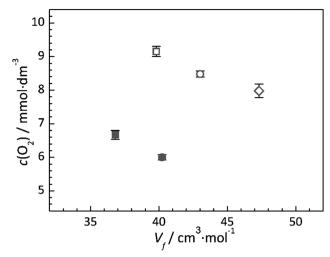
Fig. 6 Calculated IL free volume,  $V_f$ , versus the solubility of oxygen,  $c(O_2)$ , at 297 K for  $[Pyrr_{14}][TFSI]$  ( $\bigcirc$ ),  $[Pip_{14}][TFSI]$  ( $\bigcirc$ ),  $[Aze_{14}][TFSI]$  ( $\bigcirc$ ),  $[Pyrr_{1(2o_1)}][TFSI]$  ( $\bigcirc$ ). The error bars represent the standard error of the measurements.
