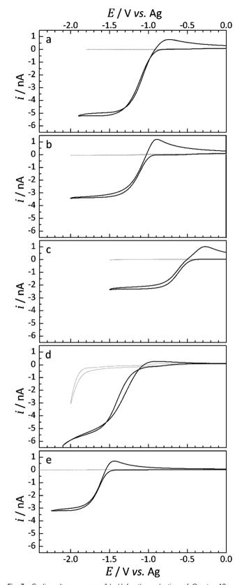
Fig. 3 Cyclic voltammograms (black) for the reduction of  $O_2$  at a 10  $\mu$ m diameter Pt-microdisk electrode vs. Ag in (a) [Pyrr<sub>14</sub>][TFSI], (b) [Pip<sub>14</sub>][TFSI], (c) [Aze<sub>14</sub>][TFSI], (d) [Pyrr<sub>1(201)</sub>][TFSI] and (e) [Pip<sub>1(201)</sub>][TFSI] at 297  $\pm$  0.5 K. The blank traces (grey) were obtained by cyclic voltammetry under an Ar atmosphere prior to exposure to  $O_2$  gas (1 barg). A scan rate of 100 mV s<sup>-1</sup> was used in all cases.
