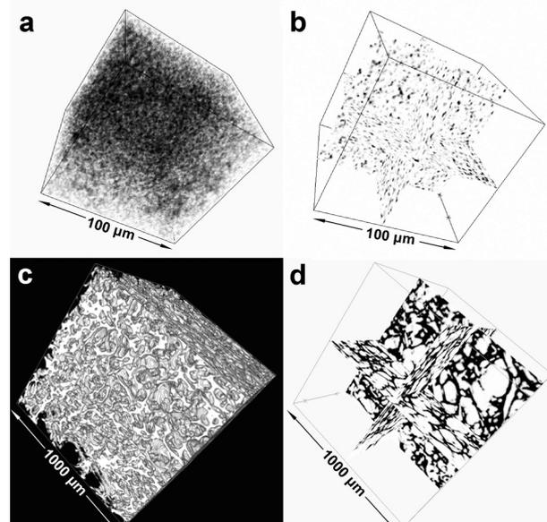
Fig. 4 3D X-ray computed tomography of the cured nanocomposite adhesive (1.0 wt%  $\text{Fe}_3\text{O}_4$  HNSs in epoxy resin) before (a & b) and after (c & d) 3 min microwave irradiation at 100 W, 2.45 GHz. (b) and (d) are the corresponding orthoslices for (a) and (c), respectively.
