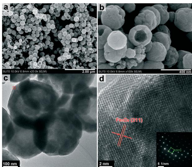
Fig. 1 FESEM (a) and (b), TEM (c) and HRTEM (d) images of as-prepared Fe<sub>3</sub>O<sub>4</sub> HNSs. Inset in Fig. 1d: corresponding SAED pattern.
