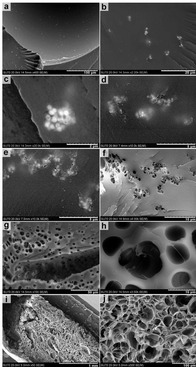
Fig. 3 FESEM images of the section structure of the cured nanocomposite adhesive sheet (1.0 wt%  $\text{Fe}_3\text{O}_4$  HNSs in epoxy resin) without microwave irradiation (a–c), with single-mode microwave irradiation at 100 W for 1 (d), 1.5 (e), 2 (f), 2.5 (g & h) and 3 (i & j) min.
