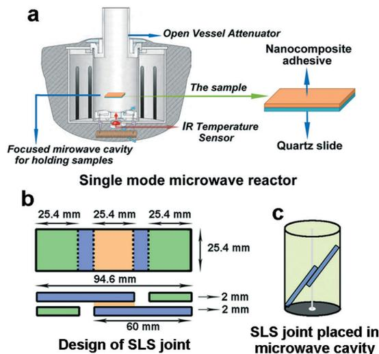
**Scheme 1** Schematic illustrations of (a) the heating procedure of cured composites (1.0 wt%  $\text{Fe}_3\text{O}_4$  HNSs in epoxy resin) in the single mode microwave reactor CEM Discover SP; (b) geometrical parameters of the SLS joint; (c) the adhesively bonded SLS joint placed in the cavity of the microwave reactor for further dielectric heating investigation.
