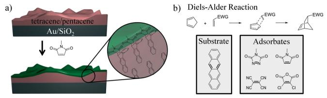
Fig. 1 (a) Schematic of the vapor based reaction of small molecules onto a sublimed tetracene or pentacene substrate. (b) Top: General mechanism for the Diels-Alder reaction ([4+2] cycloaddition). Bottom: Representative examples of the adsorbates that have been shown to successfully react with a tetracene single crystals in ref. 9. Bolded bonds indicate those involved in the reaction. EWG = electron withdrawing group.
