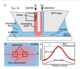
Fig. 1 Concept of hydrodynamic thermal confinement (HTC). (a) Working principle of HTC. (b) Schematic (bottom) view of heated flow confinement. (c) Graph of the temperature profile along the centerline marked in (b).
