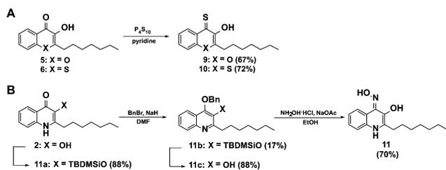
Fig. 3 Synthesis of a second generation of compounds based on the active elastase inhibitor **8**. (A) Scheme for the synthesis of the thioquinolone derivatives **9** and **10**, and (B) for the oxime **11**.
