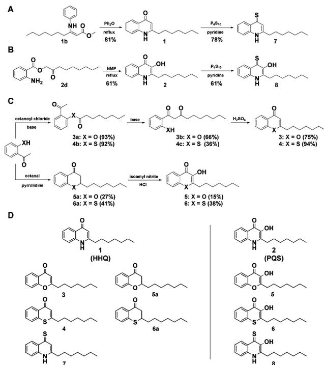
**Fig. 1** Synthetic library of HHQ and PQS derivatives. (A) Synthesis scheme for HHQ (**1**) and the derived thio-HHQ **7**, and (B) for PQS (**2**) and its analog **8**. (C) Synthesis of compounds **3–6**. (D) Structures of the compound library tested in the bioassays.
