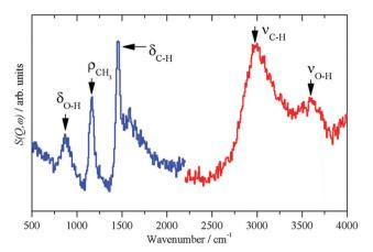
Fig. 2 INS spectrum of methoxy chemisorbed on n-alumina.
