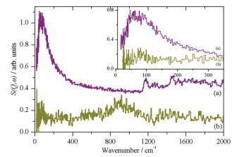
Fig. 7 INS spectra at 20 K the product of the reaction of selectively deuterated methanol with n-Al<sub>2</sub>O<sub>3</sub>: (a) CH<sub>3</sub>OD (purple) and (b) CD<sub>3</sub>OH (khaki). The inset shows the librational region on an expanded scale.
