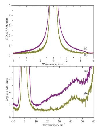
Fig. 6 QENS spectra at 2 K in a narrow (upper) and a wide (lower) energy range of the reaction products of selectively deuterated methanol with  $\eta$ -Al<sub>2</sub>O<sub>3</sub>: (a) CH<sub>3</sub>OD (purple) and (b) CD<sub>3</sub>OH (khaki).
