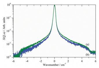
Comparison of the QENS spectra at 2 K of (a)  $\eta$ -alumina (olive) and (b) γ-alumina (blue) after reaction with methanol to generate methoxy
