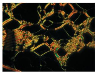
Fig. 8 Texture of the solvent induced lyotropic SmA phase of  ${\bf 1^{12}EO^3OH}$  at  $T=105~^{\circ}C$  in a mixture with ethylene glycol (EO) at  $n_{\rm EO}=10$ .
