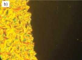
Fig. 2 Textures of  $\mathbf{1^{12}(OH)_2}$  in the (a) SmC<sub>d</sub> phase at T=167 °C and (b) in the SmA<sub>d</sub> phase at T=169 °C as observed upon heating; at the right homeotropic alignment and at the left predominately planar alignment with fan texture.
