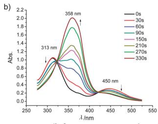
Fig. 11 UV spectra of  ${\bf 1^{12}EO^3OH}$  in CH<sub>2</sub>Cl<sub>2</sub> solution ( $c=10^{-5}$  mol L<sup>-1</sup>), changing with time: (a) from E- to Z-azobenzene under irradiation with 365 nm light; (b) from Z- to E-azobenzene under irradiation with visible light; for additional examples, see Fig. S3 and S4 (ESI†).
