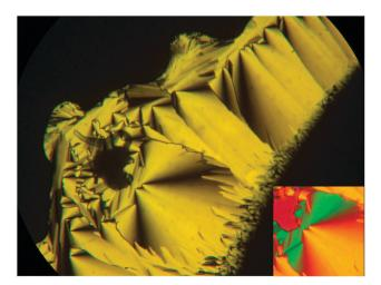
Fig. 10 Texture of the solvent stabilized lyotropic Col<sub>nex</sub> phase of  $3^{12}EO^{3}(OH)_{2}$  (right) at T = 170 °C in the contact region with formamide (left) as observed upon cooling, the inset shows the texture with the additional  $\lambda$ -plate.
