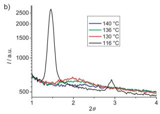
Fig. 4 Small angle XRD patterns of compounds (a) 112EO3OH and (b)  $1^{12}EO^{3}(OH)_{2}$  at the indicated temperatures in the smectic phase (black lines) and at different temperatures in the Iso phase in proximity to the SmA<sub>d</sub>-Iso transition (colored lines), showing a significant cybotaxis for 1<sup>12</sup>EO<sup>3</sup>(OH)<sub>2</sub> being much weaker for 1<sup>12</sup>EO<sup>3</sup>OH.
