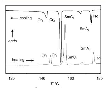
Fig. 1 DSC traces of  $1^{12}(OH)_2$  (10 K min<sup>-1</sup>).
