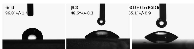
Fig. 2 Water contact angle values for gold, \beta CD monolayer and \beta CD complexed with Cb-cRGD 6 ( n = 4 ), with a representative picture. A high WCA angle value indicates a hydrophobic surface.
