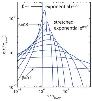
Fig. 3 Plot of the relaxation time probability density function (pdf) as a function of  $\tau/\tau_{KWW}$  where  $\tau_{KWW}$  is the relaxation time introduced in eqn (12) and (13).<sup>60</sup>  $\beta$  values range from 0.1 to ~1 to illustrate the range of relaxation distributions for sub-diffusive systems as opposed to the  $\delta$ -like distribution for Brownian diffusion (approximated by  $\beta = 0.9999$ )
