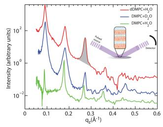
Fig. 2 Neutron diffraction data collected at the OFFSPEC reflectometer are shown for three hydrated lipid bilayer samples: (red) deuterated DMPC hydrated by  $H_2O$ , (blue) DMPC hydrated by  $D_2O$ , and (green) DMPC hydrated by  $H_2O$ . The neutron scattering length profiles in Fig. 5 were calculated from these data by using the location and areas (as shown by the shading under the peak) under each peak. All measurements were taken at  $T = 30\,^{\circ}\text{C}$  (303 K).
