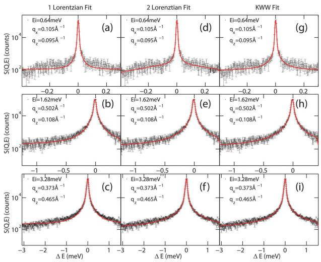
Fig. 4 Comparison between a one-Lorentzian peak fit, two-Lorentzian peak fit and Fourier transform of KWW fit of quasi-elastic broadening spectra of water diffusing in a lipid membrane. Values for  $q_x$  and  $q_z$  are indicated in each plot.
