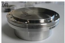
Fig. 1 Sample cans used for the neutron scattering experiments. (a) A cylindrical sample can was used for the incoherent neutron scattering experiments. (b) 18 2", 300 µm thick Si wafers were loaded into the aluminium cans. (c) Wafers were separated by 0.3 mm thick aluminum spacers to allow for hydration and the remaining space was filled with aluminum foil. (d) Sample can used for the neutron reflectivity where a single 2" wafer
