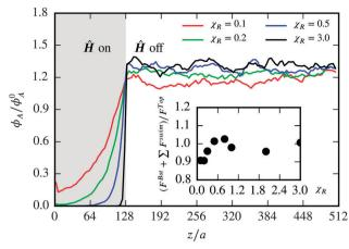
Fig. 6 A depletion zone induced by polarization. The local area fraction  $\phi_A$  vs. height z/a with the  $\hat{H}$  field applied upward in the region z < L/4 and  $\mathbf{F}^{\text{ext}} = 0$ . The solid lines are simulation. N = 1668 particles are simulated in a square box of size 512a at  $\phi_A^0$  = 0.02. The box is periodic in x but confined by no-flux walls at z = 0, L.  $Pe_R = 0.2$ ,  $D_T = a^2/\tau_R$ . The inset checks the global force balance (3) and (4).
