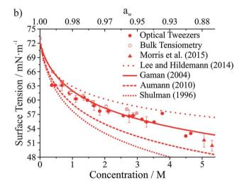
Fig. 4 Surface tension measurements on two atmospherically relevant systems: (a) sodium chloride and (b) glutaric acid. Also included are bulk tensiometry measurements, E-AIM modeling (sodium chloride), surface tension parametrizations performed by others (glutaric acid),47-50 and measurements on submicron aerosol using atomic force microscopy.<sup>28</sup> The upper axis gives water activity (a<sub>w</sub>), which is inferred from the solute concentration.
