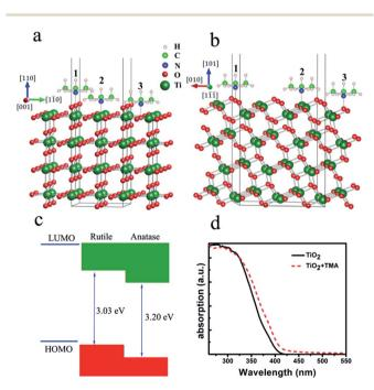
Fig. 1 The formation of a surface complex of TiO<sub>2</sub> and its implications: a and b, the possible adsorption sites of TMA onto the rutile (110) and anatase (101) surfaces of TiO2; c, schematic (not to scale) of the band alignment of TMA onto the surface of Degussa P25 TiO<sub>2</sub>; d, UV-visible absorbance spectroscopy of Degussa P25 TiO2 and the complex between TMA and TiO2.
