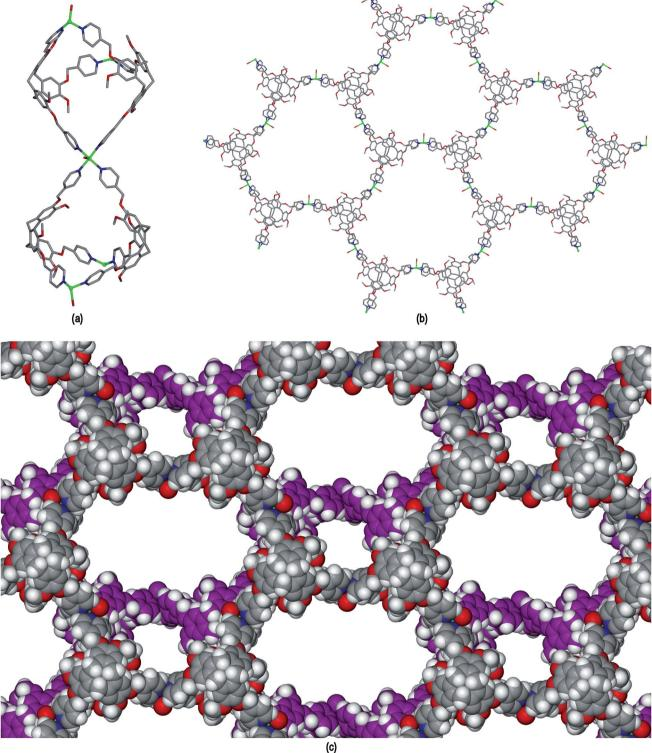
Fig. 4 From the crystal structure of  $[Cu_3(L2)_4(H_2O)_3] \cdot 6(OTf)$  2. (a) The metallo-cryptophanes of the asymmetric unit; (b) chiral 2D network of vertice-linked metallo-cryptophanes that forms in bc plane; (c) stacking of two layers of enantiomorphic 2D metallo-cryptophane layers shown in space-filling mode and in different colours for clarity.
