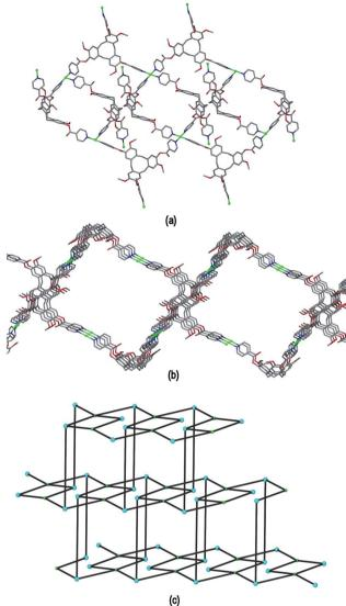
Fig. 8 From the crystal structure of  $[Cu_2(L1)_2(OTf)_2(NMP)_2(H_2O)_2]$ . 2(OTf)·2NMP 4. (a) Formation of a ladder motif through the 4-connecting Cu2 centres; (b) 2D coordination polymer of linked tubes; (c) connectivity diagram with Cu centres in green and L1 ligand centres larger spheres in blue.
