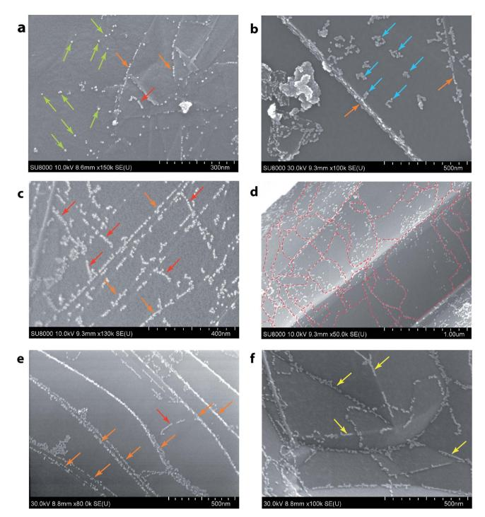
Fig. 3 Spatial imaging of different types of defects using Pd NPs. Green arrows and blue arrows indicate point defects of different sizes (a and b); red arrows indicate line defects (a, c and e); dashed red lines outline grain boundaries (d); orange arrows indicate the step edges (a-c, and e); and yellow arrows indicate topological defects (f) (see the ESI† for larger images).
