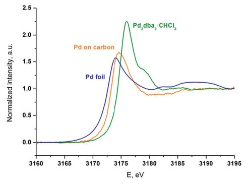
Fig. 6 XANES spectra at the Pd L<sub>III</sub> edge of the carbon material mapped with palladium NPs (orange line), the initial Pd<sub>2</sub>dba<sub>3</sub>·CHCl<sub>3</sub> (green line) and Pd foil as a standard sample (blue line).
