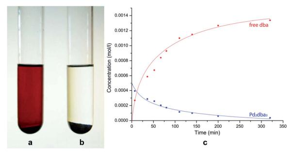
Fig. 1 Monitoring the Pd/C formation process in solution: (a) initial solution of Pd<sub>2</sub>dba<sub>3</sub> in chloroform with the added carbon material; (b) the solution after stirring for 5 h at 40 °C; (c) <sup>1</sup>H NMR monitoring of the reaction: blue line – concentration of Pd<sub>2</sub>dba<sub>3</sub>, red line – concentration of free dba.
