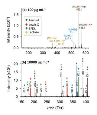
Fig. 8 Identification of oligosaccharide mixture containing lactose (brown), 3-fucosyl-p-lactose (blue), and isomeric Lewis A (green) and Lewis X (red). Full MALDI MS spectra at 100 (a) and 10 000  $\mu$ g mL<sup>-1</sup> (b) DHB@MNP. The fingerprint ions unique to 3-fucosyl-D-lactose, Lewis A and Lewis X are highlighted in blue, green and red, respectively.
