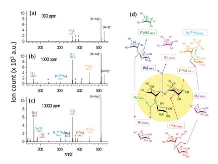
Fig. 2 Ionization behavior of 2'-fucosyl-p-lactose. (a–c) Full spectra at 300, 1000 and 10 000  $\mu$ g mL<sup>-1</sup> DHB@MNP. The DHB-derived ("\*") peaks are shown. (d) Fragmentation pattern of 2FDL. Product ion assignment is based on Domon and Costello nomenclature.<sup>36</sup>
