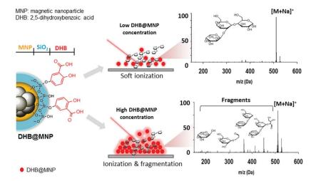
Fig. 1 Schematic representation of tunable ionization and fragmentation by nanoparticle-assisted MALDI-TOF MS for structural determination of oligosaccharides; [M + Na]<sup>+</sup> denotes sodium-adducted molecular ion peaks.
