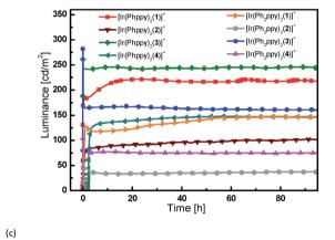
Fig. 11 Luminance vs. time for the LECs driven using pulsed current driving (a) at 300 A m $^{-2}$ , (b) at 100 A m $^{-2}$  and (c) at 50 A m $^{-2}$ , all at a frequency of 1 kHz and duty cycles of 50%.
