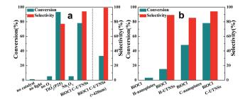
Fig. 4 Photocatalytic aerobic oxidation of 1a using different (a) semiconductor catalysts and (b) BiOCI materials. Reaction conditions: catalyst (0.077 mmol), substrate (0.1 mmol), CH<sub>3</sub>CN (4 mL), O<sub>2</sub> atmosphere, 1 h, Xe lamp irradiation.
