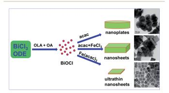
Scheme 1 Schematic illustration for the proposed formation process of BiOCI materials by a facile colloidal approach.
