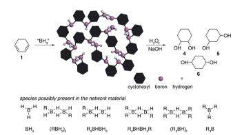
Fig. 2 Hydroboration of 1,3-cyclohexadiene 1 leading to the formation of insoluble materials which contain a range of borane species.
