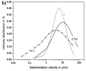
Fig. 3 Sedimentation analysis of CNT, OLC, and ND dispersion in ethylene glycol, showing (a) the sedimentation velocity of the particles as cumulative plot (including particle densities) and (b) the fitted data using a log-normal function.
