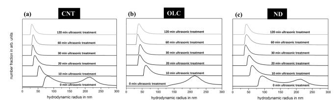
Fig. 2 DLS data of (a) CNT, (b) OLC, and (c) ND in ethylene glycol after different times of ultrasonic treatment. The spectrum of at 0 min is equal to a pre-treatment of 5 min in the homogenizer to break up the largest agglomerates.
