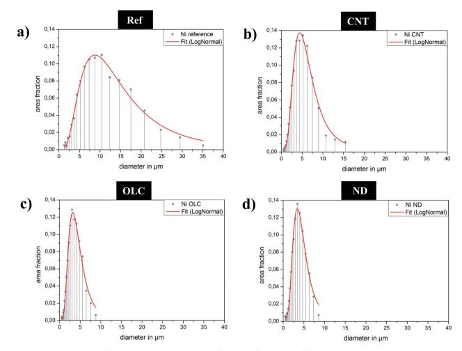
Fig. 7 Grain size distribution of (a) unreinforced nickel reference, (b) Ni CNT, (c) Ni OLC, and (d) Ni ND composites. A LogNormal fit is performed to calculate the mean grain size and the fitted curves are plotted as solid lines (red).
