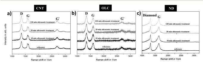
Fig. 4 Raman spectra of CNT (a), OLC (b) and ND (c) on a silicon wafer as a function of the time spent in the ultrasonic bath in the solvent ethylene glycol.
