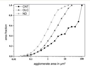
Fig. 6 Individual agglomerate area as a function of the total image agglomerate area (area fraction) in Fig. 5d-f with a resolution of 62 nm per pixel.
