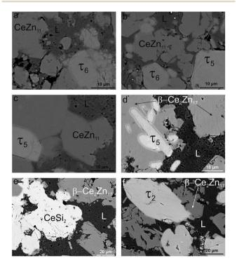
Fig. 16 Microstructure of alloy Ce $_{7.6}$ Zn $_{78.4}$ Si $_{14}$  annealed at different temperatures: (a) 650 °C, (b) 710 °C, (c) 750 °C, (d) 790 °C, (e) 880 °C, and (f) 900 °C for one day each under argon.
