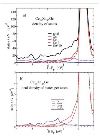
Fig. 6 Panel (a): total and local density of states (DOS) for non spinpolarized Ce<sub>7</sub>Ge<sub>0.5</sub>Zn<sub>22.5</sub>. Panel (b): local DOS per atom. For better visibility, the local DOS for Ge is multiplied by a factor of 10.
