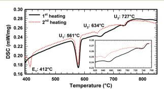
Fig. 12 DTA curve of alloy Ce<sub>5.9</sub>Zn<sub>59.8</sub>Si<sub>34.3</sub>.
