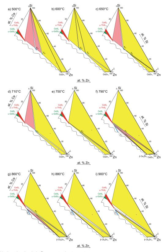
Fig. 14 Partial isothermal sections in the Zn-corner at various temperatures.
