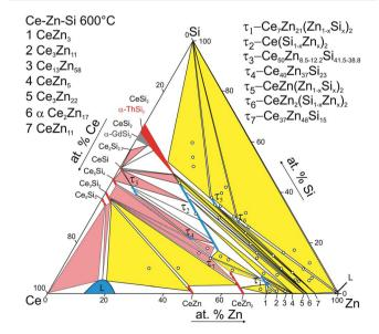
Fig. 8 Partial isothermal section at 600 °C (<33.3 at% Ce). The circles represent nominal compositions of alloys. The pink three phase fields are taken from ref. 8
