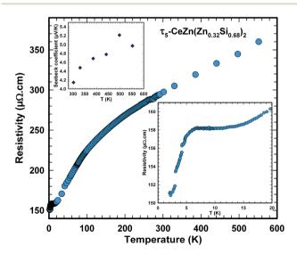
Fig. 22 Temperature dependent electrical resistivity of polycrystalline  $\tau_5$ -CeZn(Zn $_{0.32}$ Si $_{0.68}$ )<sub>2</sub>. Bottom right inset shows the kink at the ordering temperature; top left inset shows the Seebeck coefficient above room temperature.
