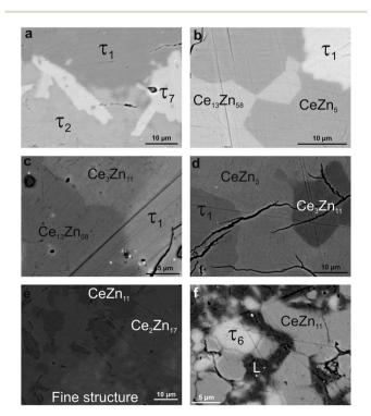
Fig. 10 Selected micrograph of Ce–Zn–Si alloys annealed at 600 °C: (a)  $Ce_{32}Zn_{54}Si_{14}$ , (b)  $Ce_{18}Zn_{81}Si_{1}$ , (c)  $Ce_{21}Zn_{78}Si_{1}$ , (d)  $Ce_{23}Zn_{76}Si_{1}$ , (e) diffusion couple  $Ce_{70}Si_{30}$ –Zn (12 hours), and (f) diffusion couple  $Ce_{50}Si_{50}$ –Zn (12 hours) (nominal composition in at.%).
