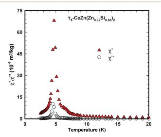
Fig. 18 Temperature dependent in-phase and out-of-phase ac susceptibility components,  $\chi'$  and  $\chi''$ , measured on polycrystalline  $\tau_5$ -CeZn(Zn<sub>0.32</sub>Si<sub>0.68</sub>)<sub>2</sub> with a field amplitude of 325 A m<sup>-1</sup> and frequency of 100 Hz.
