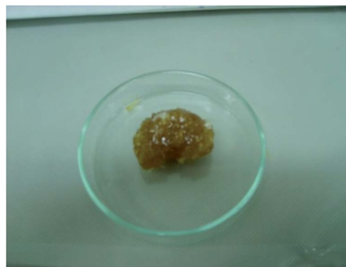
Fig. 15 Cross-linked BAMPO based epoxy sample at 120 °C.
