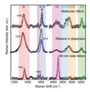
Fig. 5 Raman spectrum of an individual GNR on the Dodecvl-TESfunctionalised surface (top) compared to the spectrum of a drop of the GNR in dispersion (middle) and to that of a 100 nm wide ribbon etched from exfoliated graphene by oxygen-plasma treatment (bottom). The lines are fits to the data (see text) while the colour bars highlight the different spectral regions.
