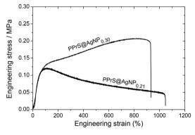
**Fig. 3** Representative engineering stress–strain curves of PPrS@AgNP $_{0.30}$  (upper curve) and PPrS@AgNP $_{0.21}$  (lower curve) from linear uniaxial tensile testing. Improved tensile strength and flow suppression is obtained with increasing  $\phi$ .
