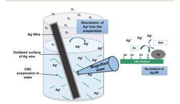
Fig. 3 Pictorial representation of the mechanism for the generation of Ag NPs from Ag wire in aqueous CNC suspensions.
