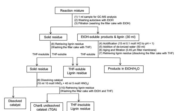
Scheme 2 Work-up procedure of reaction product mixture from lignin reaction.
