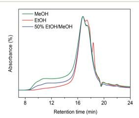
**Fig. 1** GPC chromatograms of the THF-insoluble fraction of the lignin residue following reaction in methanol, ethanol and 50%/50% (v/v) methanol/ethanol mixture at 300 °C for 4 h over the CuMgAlO<sub>x</sub> catalyst (chromatograms normalized to the total peak area).
