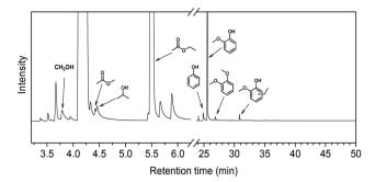
Fig. 5 GC-MS chromatograms of reaction mixtures obtained from reaction of guaiacol at 300  $^{\circ}$ C for 2 h over the CuMgAlO<sub>x</sub> catalyst in ethanol
