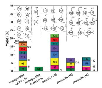
Fig. 7 Monomeric product distribution following lignin reaction at 380 °C for 8 h over the CuMgAlO<sub>x</sub> catalyst in ethanol solvent.
