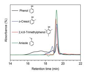
Fig. 6 GPC chromatograms of reaction mixtures obtained from the reaction at 300 °C for 1 h over the CuMgAlO<sub>x</sub> catalyst using different reactants in methanol solvent (depicted chromatograms have been normalized by the sum of the peak area).
