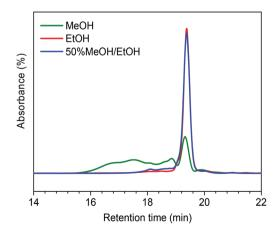
Fig. 2 GPC chromatograms of reaction mixtures obtained from the reaction of phenol at 300 °C for 1 h over the CuMgAlOx catalyst in methanol, ethanol and 50%/50% (v/v) methanol/ethanol mixture (chromatograms normalized to total peak area).
