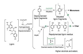
Scheme 1 The roles of alkylation, the Guerbet reaction, and esterification on suppressing char formation during lignin depolymerization over the CuMgAlO<sub>x</sub> catalyst in supercritical ethanol.
