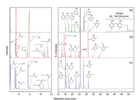
Fig. 3 GC-MS chromatograms of reaction mixtures obtained from reaction of phenol at 300 °C for 1 h over the CuMgAlO<sub>x</sub> catalyst in (a) methanol, (b) ethanol, and (c) 50%/50% (v/v) methanol/ethanol solvents (GC-MS chromatograms normalized to the internal standard, ISTD).
