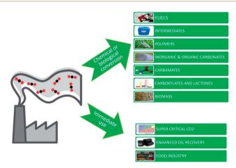
Fig. 1 Some products that CO<sub>2</sub> can be converted to *via* carbon dioxide utilisation (CDU) processes. Source: CO2Chem Network, available at http://www.co2chem.co.uk. Reproduced with the permission of CO2Chem Media and Publishing Limited.
