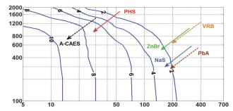
Fig. 4 Market share of BES (% of load supply) with a carbon cap of 150 kgCO<sub>2</sub>e per MW h. Horizontal and vertical axes indicate  $X_E$  (\$ per kW h) and  $X_P$  (\$ per kW). Arrows start from the current cost estimates (average of the range shown for each technology in Fig. 1) and end at points with 50% reduction in both  $X_E$  and  $X_P$ .
