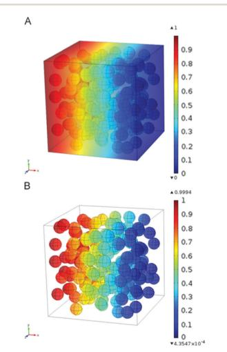
Fig. 4 Concentration profiles of (a) both matrix and filler domains, and (b) filler domain only, of a membrane model with randomly distributed filler. Length units are in µm and concentration in mol m<sup>-1.75</sup> Reproduced with permission from Elsevier.
