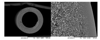
SEM images of the cross section of a polysulfone hollow fiber membrane, (a) overall, (b) outer edge
