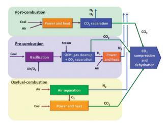
Fig. 1 Technical options for CO<sub>2</sub> capture from coal-power plants.<sup>1</sup>
