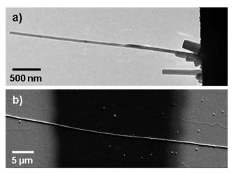
Fig. 1 Individual Aq-TCNQ wires for microscopic and spectroscopic investigations in operando. (a) Transmission electron micrograph of an Ag-TCNQ nanowire (d = 41 nm) on a gold support, which can be contacted with a tungsten tip in the TEM. (b) Scanning electron micrograph of a crystallite (d =0.35 µm) contacted with gold electrodes (the brighter areas on both sides).
