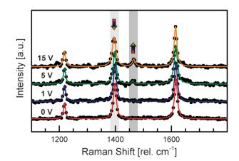
Fig. 3 Reverse charge transfer probed using Raman spectroscopy. Raman spectra of an individual Ag-TCNQ wire under operation. With an increase in negative voltage (absolute values shown), the typical band for neutral TCNQ arises at 1457 rel. cm<sup>-1</sup> whereas the vibration of the negative molecule at 1388 rel. cm<sup>-1</sup> is diminished.
