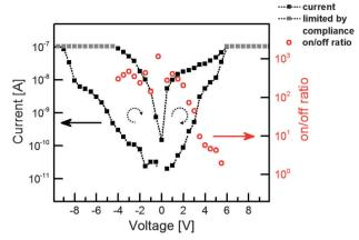
Fig. 2 Current-voltage characteristics of an individual Ag-TCNQ crystallite. Negative and positive dual voltage sweeps have been conducted: 0 V  $\rightarrow$  $-10 \text{ V} \rightarrow 10 \text{ V} \rightarrow 0 \text{ V}$  (black, squares). The on/off-ratios well exceed  $10^2$ (red, open circles). The on/off-ratios in the regime with limited current flow by the chosen compliance value (grey squares) cannot be determined and are therefore not shown.
