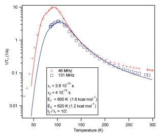
Fig. 3 Variable-temperature proton spin-lattice relaxation time, <sup>1</sup>H  $T_1^{-1}$ , at two fields for 1.
