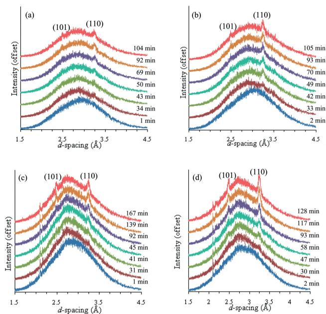
Fig. 1 In situ EDXRD data collected during the hydrothermal synthesis of TiO2 nanoparticles from HNO3 peptized sol-gels at (a) 210 °C, (b) 230 °C, (c) 250 °C and (d) 270 °C. Modified versions of our previously published EDXRD graphs.<sup>50</sup>
