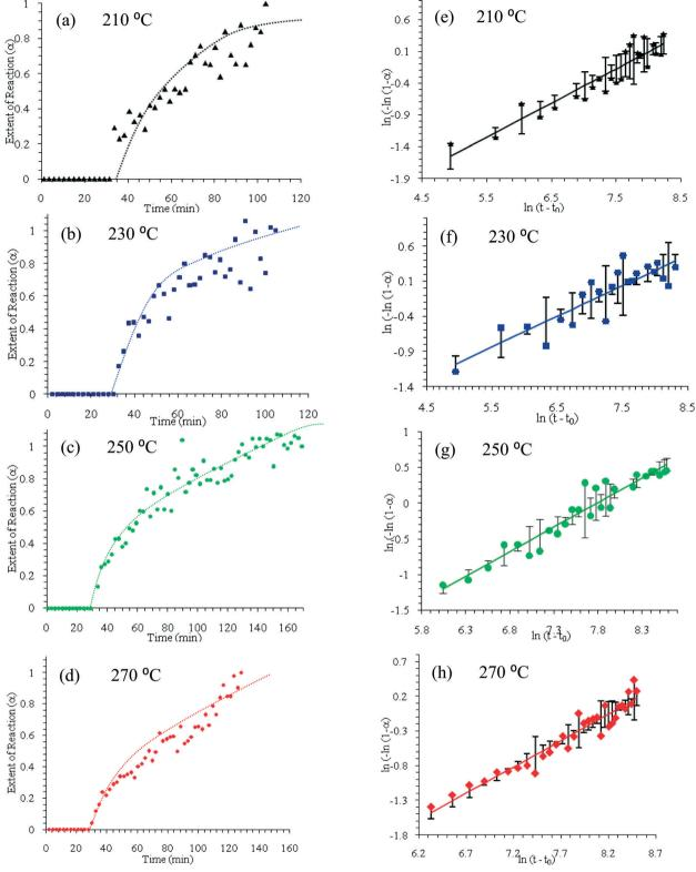
Fig. 2 Extent of reaction against time for the (110) peak of  $TiO_2$  particles produced by *in situ* hydrothermal processes at 210, 230, 250 and 270 °C (a–d) and their corresponding Sharp and Hancock plots showing the kinetic data (e–h), respectively.
