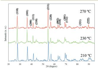
Fig. 3 XRD patterns of  $\rm TiO_2$  nanoparticles produced by in situ hydrothermal reactions of HNO $_3$  peptized sol-gels at 210 °C, 230 °C and 270 °C. Modified versions of our previously published XRD patterns  $^{50}$
