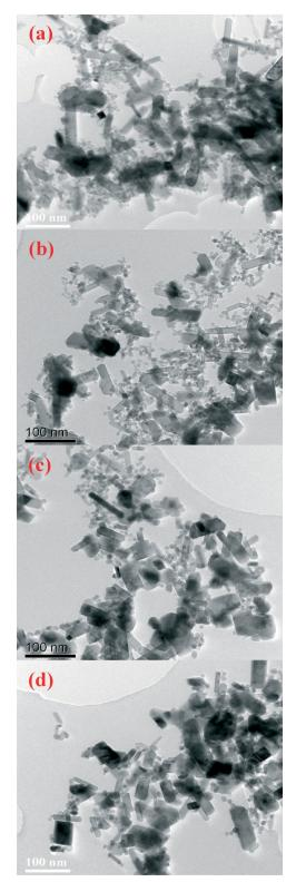
Fig. 4 TEM images of  $TiO_2$  nanoparticles produced by in situ hydrothermal reactions of  $HNO_3$  peptized sol-gels at (a) 210 °C, (b) 230 °C, (c) 250 °C and (d) 270 °C.
