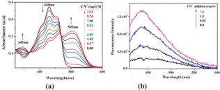
Fig. 4 (a), UV/Vis titration profile of  $\mathbf{1}$  (20.6  $\times$  10<sup>-6</sup> M) upon addition of NaCN (0.3 mM) in DMSO/HEPES (8:2, v/v). (b) Emission response of 1  $(7.5 \times 10^{-6} \text{ M})$  with NaCN in DMSO/HEPES (8:2, v/v) upon excitation at 390 nm. All these experiments were carried out at 298 K.
