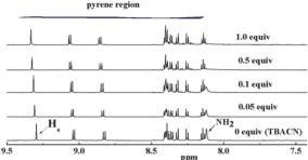
Fig. 5 Complete <sup>1</sup>H NMR of **1** (25 mM) in d<sub>6</sub>-DMSO with TBACN (2 mM) in THF. The experiment was carried out at 298 K.
