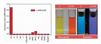
Fig. 3 (left) Bar graph presenting high selectivity of 1 for CN<sup>-</sup>. Observations were made by addition of 7.0 equivalents of sodium cyanide (NaCN, 0.3 mM) in water to 1 (20.6  $\times$  10<sup>6</sup> M) in DMSO. Other anions were used in 100-fold concentrations. (right) Visual display of CN<sup>-</sup> mediated PTS in absorption and emission mode
