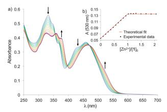
Fig. 3 (a) UV-Vis titration of tweezers  $\mathbf{1}$  (5.0  $\times$  10<sup>-6</sup> mol L<sup>-1</sup>) with Zn(ClO<sub>4</sub>)<sub>2</sub> in CHCl<sub>3</sub>. (b) Absorption at 530 nm and fitting with a 1:1 binding model.
