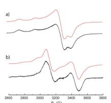
Fig. 5 X-band EPR spectrum of (a) open tweezers  $\mathbf{1}$  and (b) closed tweezers  $[Zn(\mathbf{1})](ClO_4)_2$  in frozen solution of CHCl<sub>3</sub>  $(1.0 \times 10^{-4} \text{ mol L}^{-1})$  at 5 K (black): theoretical fit (red).
