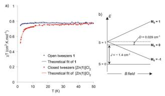
Fig. 6 (a)  $\chi T = f(T)$  of open tweezers 1 (blue), and closed tweezers  $[Zn(1)]Cl_2$  (red), in the solid state; experimental points, and theoretical fit (plain); (b) energy level diagram of the spin system.
