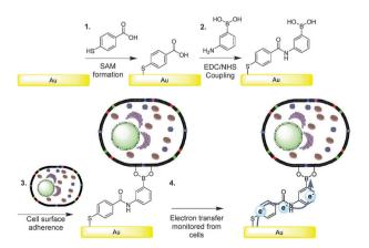
Fig. 1 Schematic representation of (1) the formation of the carboxylic acid-terminated SAM, (2) the coupling of 3-aminophenylboronic acid and (3) the binding of cells *via* cyclic boronic ester formation. (4) Charge transfer events from cells enabled by the fabrication of electrodes with boronic acid (BA)-terminated self-assembled monolayers (SAMs).
