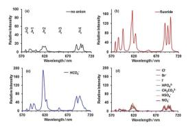
**Fig. 2** Comparison of the emission spectrum of (a) **[Eu.L¹]**<sup>+</sup> with the limiting emission spectra of **[Eu.L¹]**<sup>+</sup> in the presence of: (b) 2 mM fluoride; (c) 2 mM HCO<sub>3</sub>; and (d) 2 mM Cl<sup>-</sup>, Br<sup>-</sup>, I<sup>-</sup>, HPO<sub>4</sub><sup>2-</sup>, CH<sub>3</sub>CO<sub>2</sub><sup>-</sup>, HSO<sub>4</sub><sup>-</sup>, NO<sub>3</sub><sup>-</sup> (sodium salts). Conditions: H<sub>2</sub>O (25 mM HEPES, pH 7.4),  $\lambda_{\text{exc}}$  = 332 nm, 298 K.
