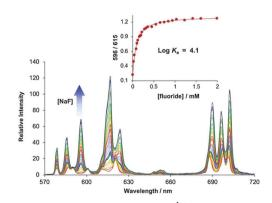
Fig. 3 Change in emission spectra of [Eu.L¹]+ (20  $\mu$ M) as a function of added NaF. Conditions: H<sub>2</sub>O (25 mM MES, pH 6.0),  $\lambda_{exc}$  = 332 nm, 298 K. The inset shows the fit to the experimental data, for log  $K_a$  = 4.1 (±0.1).
