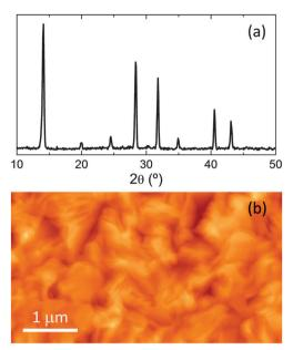
Fig. 2 (a) GIXRD pattern and (b) AFM topography of a CH<sub>3</sub>NH<sub>3</sub>Pbl<sub>3</sub> thin film deposited by flash evaporation.
