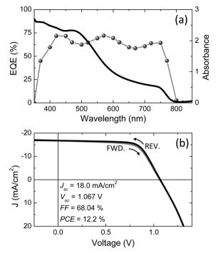
Fig. 3 (a) EQE (symbols) and optical absorption (line) in the UV-visible region for a planar perovskite solar cell and its active layer, respectively, deposited by flash evaporation. (b) J-V curve in forward (FWD.) and reverse (REV.) bias for a device under illumination with the structure ITO/PEDOT:PSS/polyTPD/MAPbl $_3$ /PCBM/Ba/Ag. The scan rate in both bias direction was 0.1 V s $^{-1}$ .
