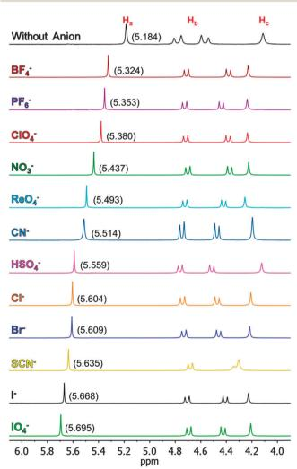
Fig. 2  $^{1}$ H NMR spectra (500 MHz, 5%  $D_{2}O-DMSO-d_{6}$ , 30  $^{\circ}$ C, TMS) of **BU-1**  $(c_{(BU-1)} = 1 \times 10^{-3} \text{ M})$  in the absence and presence of 12 anions (in excess). The chemical shifts of the Ha signals in each spectrum are given in brackets. Anions were added in the form of tetrabutylammonium (TBA) salts.
