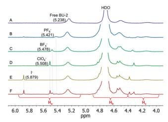
Fig. 5  $\,^{1}$ H NMR spectra (500 MHz, D<sub>2</sub>O, 20 mM K<sub>2</sub>DPO<sub>4</sub>, 30  $\,^{\circ}$ C) of **BU-2**: (A) in the absence of an anion, (B–E) in the presence of specific anions, and (F) in the presence of 4 anions. Concentrations of anions ( $c_{(A)} = 1.0 \times 10^{-5}$  M) and the macrocycle ( $c_{(BU-2)} = 1.0 \times 10^{-3}$  M) were kept constant for all experiments. The chemical shifts of the H<sub>a</sub> signals in each spectrum are given in brackets.
