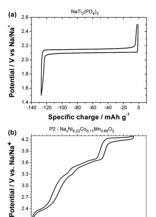
**Fig. 1** Potential profile of (a) carbon coated (2 wt%) NaTi $_2$ (PO $_4$ ) and (b) P2-type Na $_x$ Ni $_{0.22}$ Co $_{0.11}$ Mn $_{0.66}$ O $_2$  in the second cycle at 0.1C (12 mA g $^{-1}$ ) as solid electrodes. Electrolyte solutions: (a) 1 M NaClO $_4$  in PC, (b) 1 M NaPF $_6$  in PC. Three-electrode Swagelok cell in which the counter and reference electrode was metallic sodium. Temperature: 22 °C.
