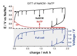
Fig. 2 GITT potential curves of the SSFB consisting of suspensions of P2-type  $Na_xNi_{0.22}Co_{0.11}Mn_{0.66}O_2-C/NaTi_2(PO_4)_3$  (positive and negative electrodes, respectively) at 0.5 mA cm $^{-2}$  (ca. 0.35 C) in static. The upper part displays the potentials profiles of the positive and negative electrode versus a reference of Na/Na $^+$ , and the bottom part depicts the resulting voltage of the battery.
