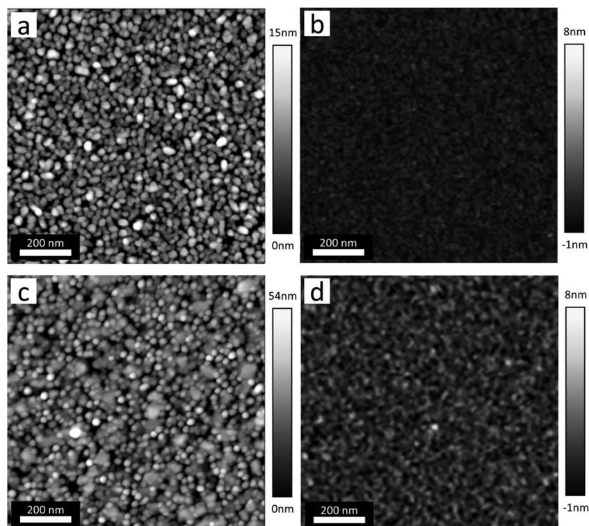
Fig. 5 AFM topography images. (a) 4 nm PTCDA on SiO<sub>2</sub>/Si. (b) 25 nm Co on SiO<sub>2</sub>/Si. (c) 18 nm TbPc<sub>2</sub> on PTCDA. (d) 18 nm TbPc<sub>2</sub> on Co.
