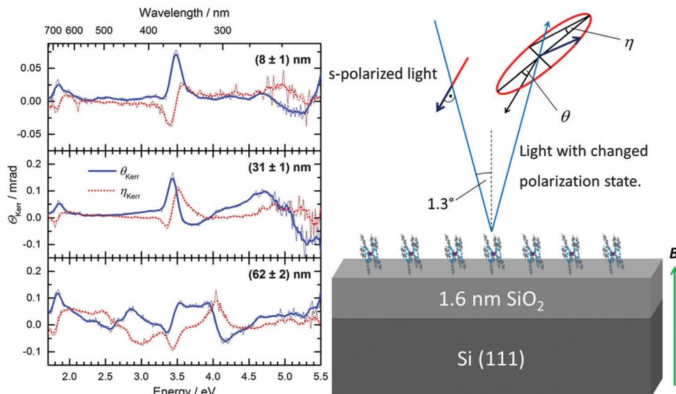
Fig. 1 (left) MOKE spectra of TbPc<sub>2</sub> films with three different thicknesses grown on SiO<sub>2</sub>/Si. The continuous lines (blue online) and dotted lines (red online) represent the spectra of the Kerr rotation and the Kerr ellipticity, respectively. The experimental data were averaged over five neighbouring points using the Boxcar filter. (right) Sketch of the measurement geometry.
