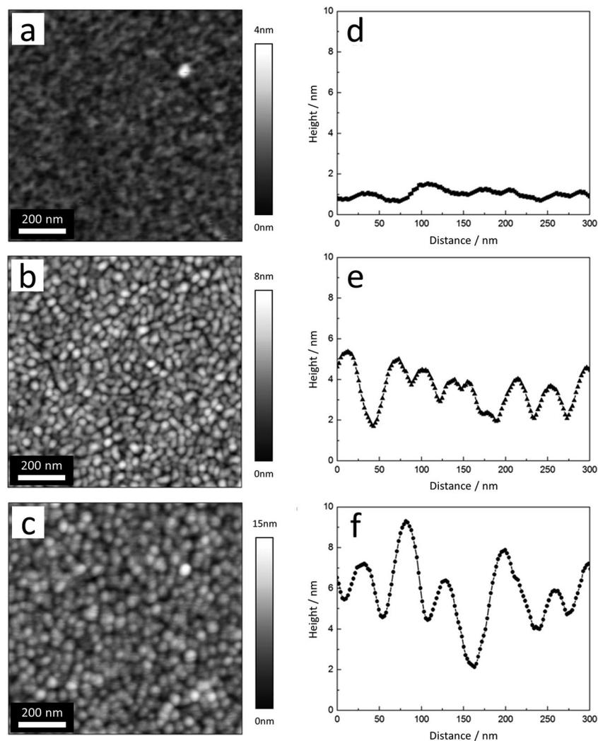
Fig. 4 (a–c) AFM topography images and (d–f) typical line profiles of TbPc<sub>2</sub> films with average film thicknesses of (a and d) 8 nm, (b and e) 31 nm, and (c and f) 62 nm.
