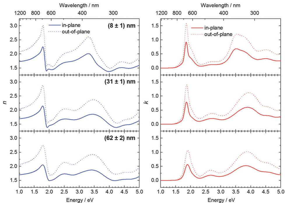
Fig. 2 Real part of the refractive index (left) and the extinction coefficient (right) of TbPc<sub>2</sub> thin films with different thicknesses.
