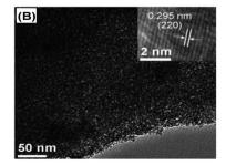
Fig. 7 (A) Schematic diagram showing the synthesis steps of preparing mesoporous ZnGa<sub>2</sub>O<sub>4</sub> through mesoporous colloidal template and ion-exchange reaction and (B) TEM image of the resulting mesoporous ZnGa<sub>2</sub>O<sub>4</sub> (inset: HR-TEM image of the crystal fringes). Reproduced with permission from ref. 113. Copyright 2010 Wiley.
