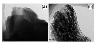
Fig. 9 TEM images of (a) non-porous g- $C_3N_4$ , and (b) porous p-g- $C_3N_4$ . Reproduced from ref. 119 with permission from The Royal Society of Chemistry.
