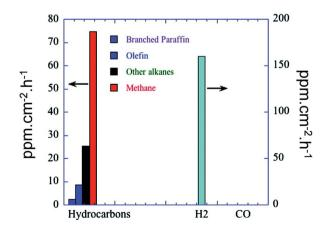
Fig. 5 Product formation of N-doped TiO<sub>2</sub> NTs arrays, calcined and sputtered coated with Pt and Cu. CO<sub>2</sub> photoreduction was conducted in a batch reactor under natural sunlight illumination in the presence of water vapour at 44 °C. Reprinted with permission from ref. 40. Copyright 2009 American Chemical Society.
