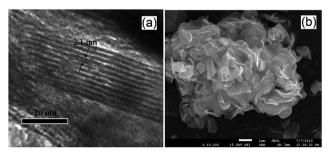
Fig. 11 (a) TEM and (b) SEM images of  $SiO_2$ -pillared  $HNb_3O_8$ . Reprinted with permission from ref. 129. Copyright 2009 American Chemical Society.
