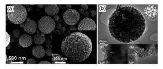
Fig. 8 (a) FE-SEM and (b) TEM and HR-TEM images of mesoporous  $TiO_2 - SiO_2$  composites prepared at 800 °C. Reproduced from ref. 108 with permission from The Royal Society of Chemistry.
