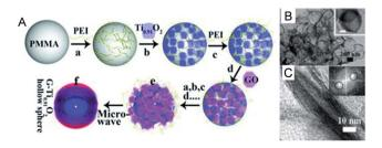
Fig. 23 (A) Stepwise preparation of alternating  $TiO_2$  and graphene nanosheet hollow sphere assemblies, (B) TEM and (C) and HR-TEM images of  $(G-Ti_0O_2)_5$  hollow spheres. Scale bar of the inset in (c): 100 nm. Inset in (C) is the fast Fourier Transform pattern of the ordered lamellar structures exhibited by the  $(G-Ti_{0.91}O_2)_5$  hollow spheres. Reproduced with permission from ref. 210. Copyright 2012 Wiley.
