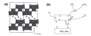
Fig. 10 Schematic depicting (a) the layered structure of  $HNb_3O_8$ , and (b) proposed mechanism of  $CO_2$  photoreduction over  $HNb_3O_8$ . Reprinted from ref. 128, Copyright 2012, with permission from Elsevier.
