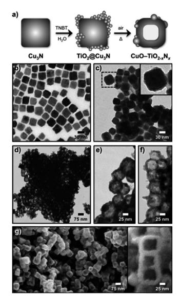
Fig. 17 (a) Schematic for the synthesis of hollow  $CuO-TiO_{2-x}N_x$ hybrid nanocubes, and associated TEM images of (b) Cu<sub>3</sub>N nanocubes, (c)  $TiO_2@Cu_3N$  nanocubes, (d)-(f) hollow  $CuO-TiO_{2-x}N_x$  hybrid nanocubes at different magnifications, and (g)-(h) FESEM images of the hollow hybrid nanocubes. Reproduced with permission from ref. 168. Copyright 2012 Wiley.
