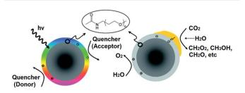
Fig. 20 PEG-functionalised carbon nanoparticles undergoing radiative recombination (left) and noble metal-coated & PEG-functionalised carbon nanoparticles photoreducing CO<sub>2</sub> (right). Reprinted with permission from ref. 184. Copyright 2011 American Chemical Society.
