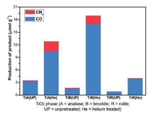
Fig. 2 CH<sub>4</sub> and CO productivity from untreated and He-treated TiO<sub>2</sub> polymorphs during 6 h illumination under 150 W solar simulator in the presence of CO<sub>2</sub>/H<sub>2</sub>O vapour, in a continuous-flow mode photoreactor operating at a flow rate of 2 mL min<sup>-1</sup>. Reprinted with permission from ref. 80. Copyright 2012 American Chemical Society.
