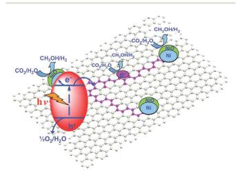
Fig. 22 Schematic of potential pathways for the transport of photo-induced electrons from a  ${\rm Ta_2O_5}$  semiconductor nanoparticle to active  ${\rm CO_2}$  photoreduction sites mediated by graphene. Reproduced from ref. 207 with permission from The Royal Society of Chemistry.
