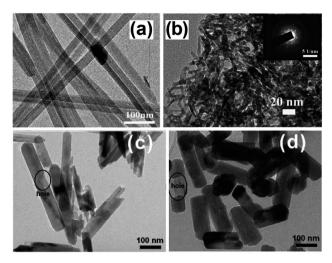
Fig. 4 TEM images of (a)  $\rm Zn_2GeO_4$  nanoribbons<sup>94</sup> and (b)  $\rm In_2Ge_2O_7$ sub-nanowires (inset: corresponding SAED pattern)96 prepared by solvothermal treatment using a binary ethylenediamine/water solvent system, and Zn<sub>2</sub>GeO<sub>4</sub> sub-nanowires prepared through solution phase route (c) at 40 °C and (d) 100 °C. Reproduced from ref. 97 with permission from The Royal Society of Chemistry.
