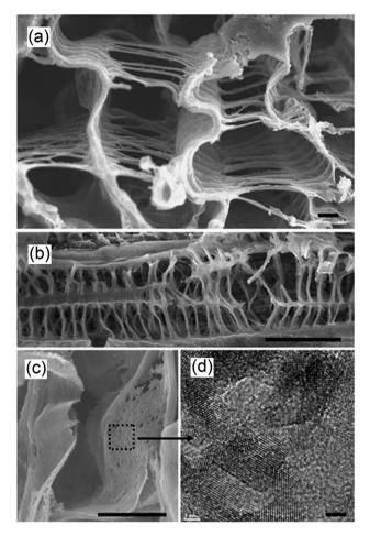
Fig. 15 FE-SEM images showing (a) the cross section of the porous venation architecture of SrTiO<sub>3</sub> (scale bar, 1 μm) (b) cross section of the porous network axially (scale bar, 10 µm), (c) magnified image of the wall of the network (scale bar, 1 µm) and (d) TEM image showing the mesoporous structure of SrTiO<sub>3</sub> (scale bar, 2 nm). Reprinted by permission from Macmillan Publishers Ltd ref. 158, copyright 2013.
