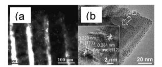
Fig. 24 (a) Dark field (S)TEM image of ultrafine Pt NPs deposited TiO<sub>2</sub> nanotube arrays,<sup>220</sup> and (b) TEM image of size resolved ultrafine Pt NPs on TiO2 film. Inset: HRTEM image showing the lattice fringes corresponding to anatase TiO<sub>2</sub> (112) and Pt (111) NPs. Reproduced from ref. 157 with permission from The Royal Society of Chemistry.
