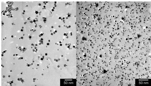
Fig. 1 As-prepared Pt nanoparticles deposited from aqueous colloids. (Left) Cubic Pt nanoparticles prepared by  $\text{H}_2$  reduction of  $[\text{Pt}(\text{OH})_6]^{2-}$  at pH 9.7. Note the presence of a minority of tetrahedra and cubo-octahedra. (Right) Tetrahedral Pt nanoparticles prepared by  $\text{H}_2$  reduction of  $[\text{Pt}(\text{OH})_6]^{2-}$  at pH 10. Many truncated tetrahedra are present, but cubes are rare.
