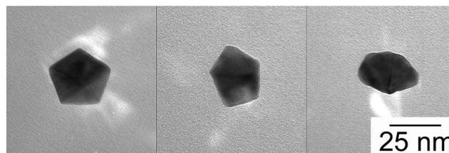
Fig. 5 Three views, at different angles of TEM stage tilt, of a particularly large decahedron formed by reduction of  $[\text{Pt}(\text{OH})_6]^{2-}$  with borohydride ion.
