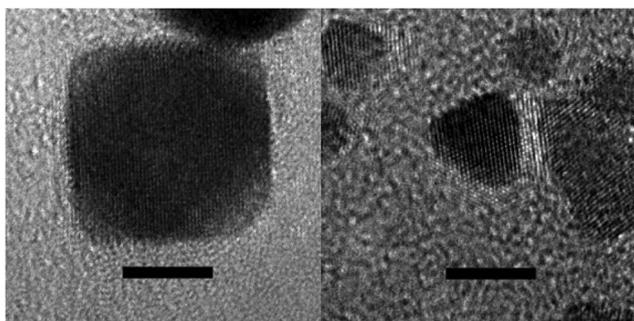
Fig. 2 High-resolution TEM images of a typical cubic Pt nanoparticle (left image) and of a typical tetrahedral Pt nanoparticle (right image). Scale bars = 5 nm.
